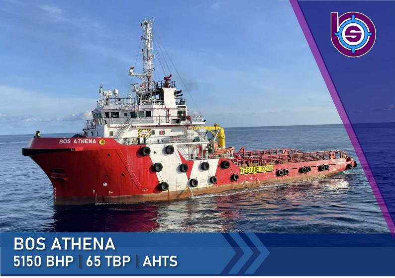
**Class Notation:** LR 100A1 AHTS, Fire-Fighting Ship 1 (2,400 m3/h) with Water Spray
